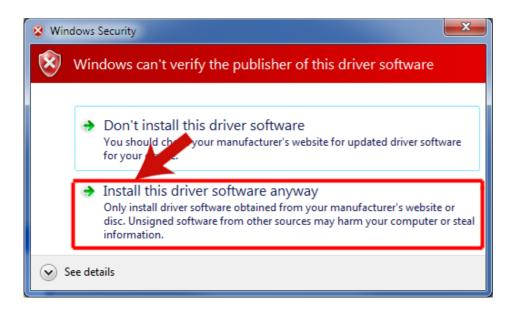
When the CNC USB Controller is connected to the USB Port, Windows 7 will detect controller hardware and begin the driver installation process. 'Windows Security' will launch a 'publisher verification' request.
