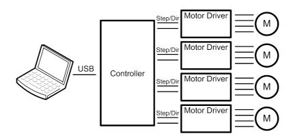
The PlanetCNC series of USB CNC motion controllers are link between a personal computer and motor drivers supporting step/direction control. They are compatible with most drivers. The controllers use the USB port, available on all modern computers and laptops. They can serve as direct replacement or upgrade for many parallel port break-out boards.
